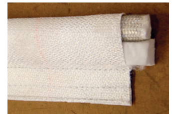
Tadpole seal fabricated from Nextel ceramic fabric*
